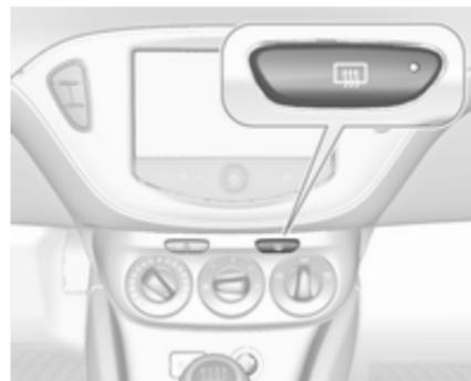
Per inserire il riscaldamento premere il pulsante
